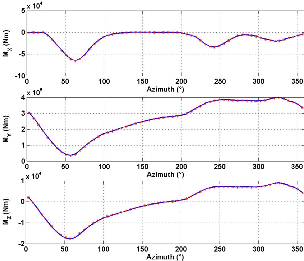
Figure 8: Comparison of the internal moments computed by NeSToR (red stars) and a commercial beam-element model (blue line). Results are presented in a cylindrical coordinate system rotating with the blade. (x: radial, y: orthoradial, z: vertical).
