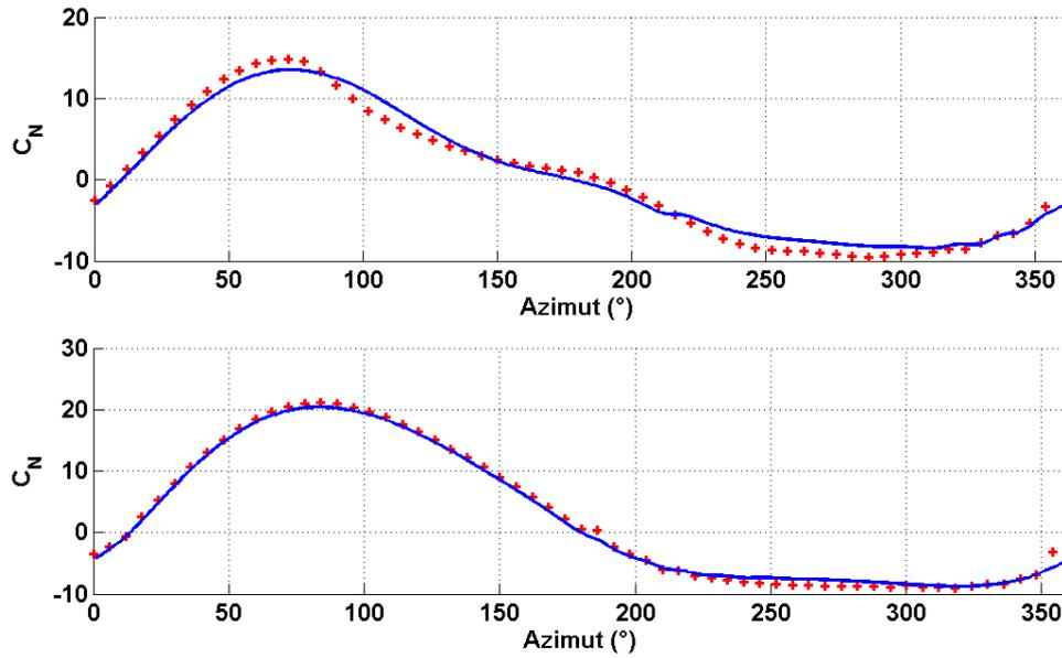
Figure 4: Normal aerodynamic coefficients of the 1HS blades over one rotation at low TSR (top) and high TSR (bottom). Comparison between PHARWEN (red cross) and CFD 2D (blue line).
