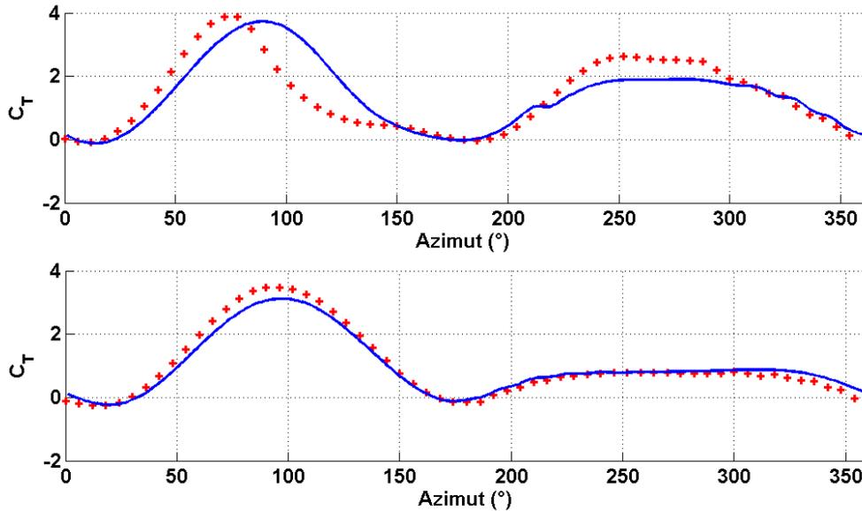
Figure 5: Tangential aerodynamic coefficients of the 1HS blades over one rotation at low TSR (top) and high TSR (bottom). Comparison between PHARWEN (red cross) and CFD 2D (blue line).
