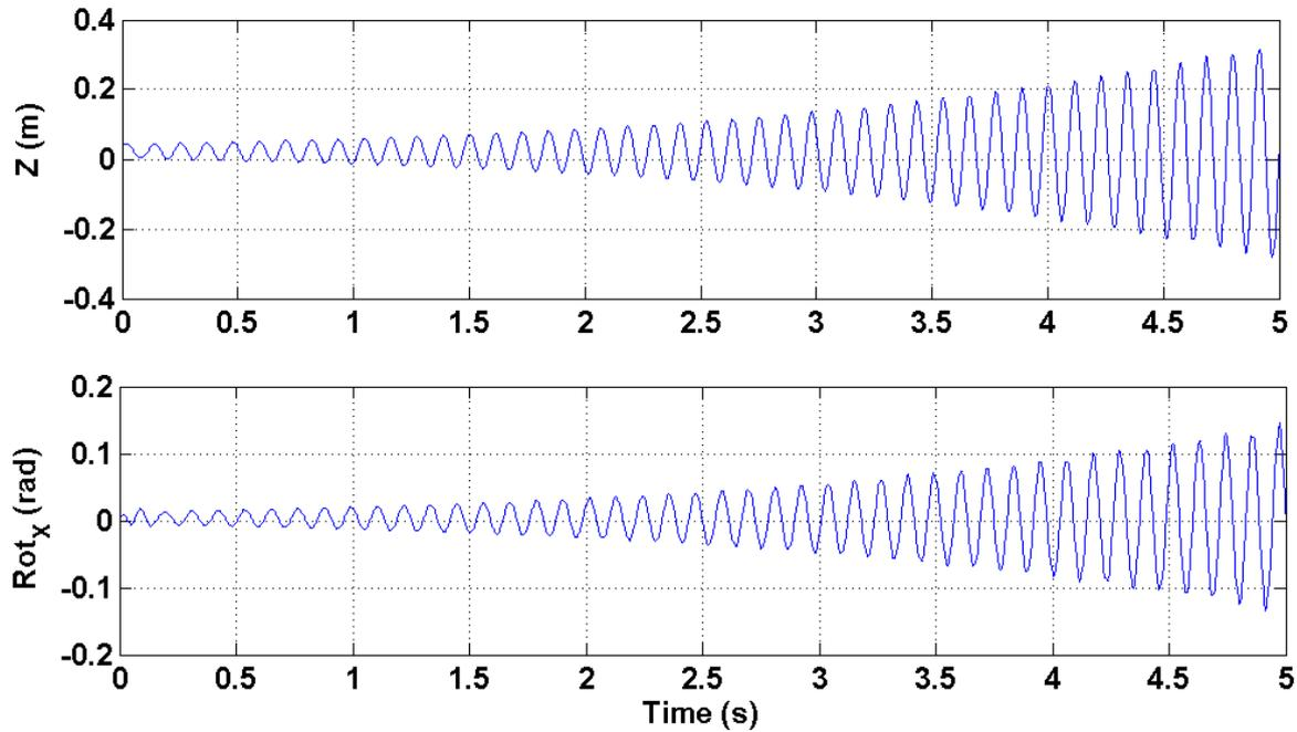
Figure 9: Bending displacement and torsion of the blade tip at a wind speed of 150 m/s
