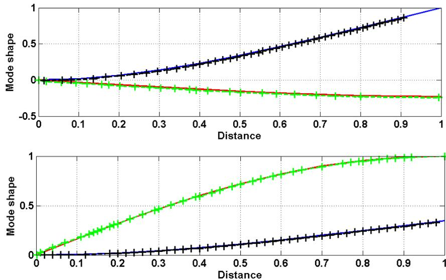
**Figure 6: Comparison of the mode shapes between NeSToR (plain lines) and [14] (cross lines). Mode 1(top) shows a predominance of bending (blue and black lines) while Mode 2 (bottom) shows a predominance of torsion (red and green lines).**
