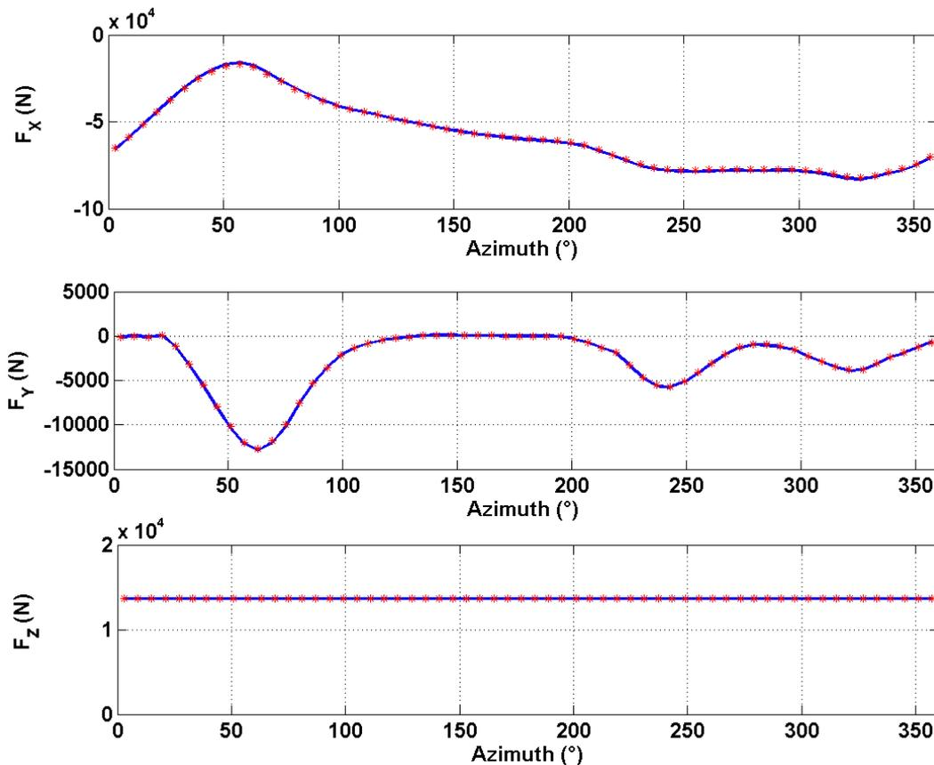
Figure 7: Comparison of the internal forces computed by NeSToR (red stars) and a commercial beam-element model (blue line). Results are presented in a cylindrical coordinate system rotating with the blade. (x: radial, y: orthoradial, z: vertical).
