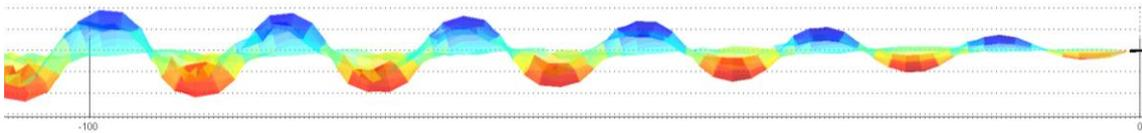
Figure 10: Wake of the Golang wing at a wind speed of 150 m/s. Side view. The wind is coming from the right.
